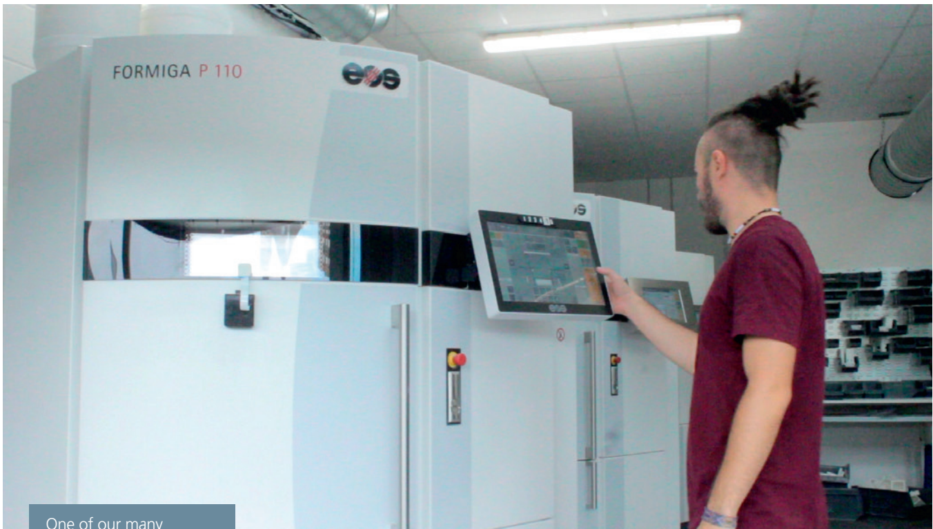
One of our many state-of-the-art SLS 3D printers being started
