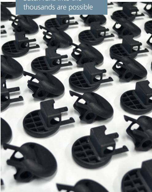
Highly complex engineering parts can be made in low volumes much cheaper than other manufacturing technologies
